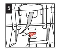
Insert metal clip up through the shell and pad.
